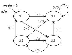
It is a Mealy FSM as the output depends on the input as well as the present state.
